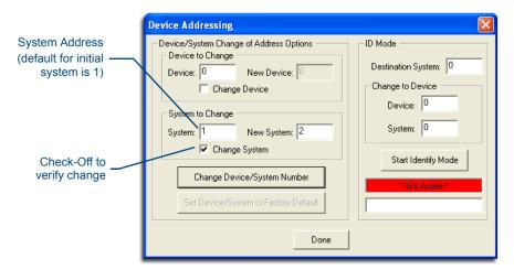
FIG. 16 Device Addressing tab (changing the system value)
